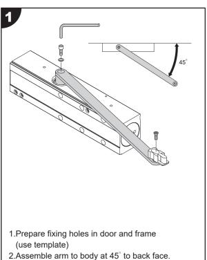
Secure arm and sliding block with bolts provided.
