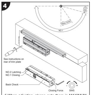
5.When adjusting, please note there is MAXIMUM of 2 TURNS for Latching, Closing and Back Check valves. Over adjustment will affect the performance of the closer. for the number of turns required to adjust the closing force, please refer to the table below.
